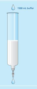
Check to ensure the stopcock is in the open position. Place a suitable waste reservoir at the outlet.
