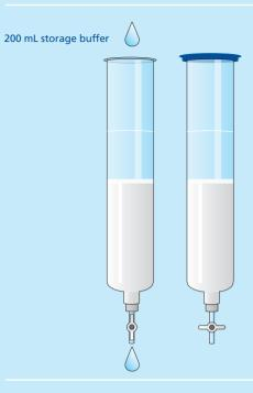
For storage, prepare a buffer containing one of the following: 20% ethanol in water, 0.02% sodium azide in water, or 0.15% ProClin in water. Allow 1500 mL of storage buffer to flow through the column. Discard the eluent\*. Add an additional 200 mL of storage buffer, close the stopcock, and reseal the blue upper cap onto the top of the column.
