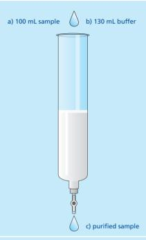
Carefully and evenly transfer a 100 mL sample onto the top of the upper frit. Allow the sample to completely enter the gel bed. Some eluent will flow out of the column and this can be discarded.
