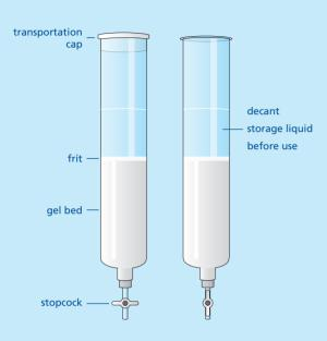
Allow the column to warm to ambient temperature if it has been refrigerated. Check to ensure the stopcock is in the closed position. Carefully remove the transparent transportation cap from the top of the CentriPure N1000 column and decant the storage liquid above the upper frit into a suitable waste reservoir.\*
