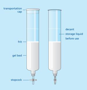
Allow the column to warm to ambient temperature if it has been refrigerated. Check to ensure the stopcock is in the closed position. Carefully remove the transparent transportation cap from the top of the CentriPure N200 column and decant the storage liquid above the upper frit into a suitable waste reservoir.\*
