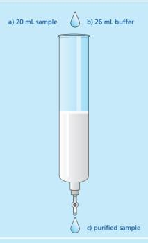
Carefully and evenly transfer a 20 mL sample onto the top of the upper frit. Allow the sample to completely enter the gel bed. Some eluent will flow out of the column and this can be discarded.
