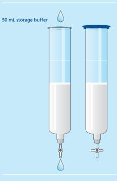
For storage, prepare a buffer containing one of the following: 20% ethanol in water, 0.02% sodium azide in water, or 0.15% ProClin in water. Allow 300 mL of storage buffer to flow through the column. Discard the eluent\*. Add an additional 50 mL of storage buffer, close the stopcock, and reseal the blue upper cap onto the top of the column.
