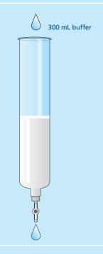
Check to ensure the stopcock is in the open position.
