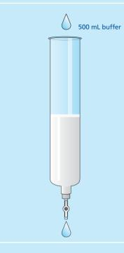
Check to ensure the stopcock is in the open position. Place a suitable waste reservoir at the outlet.
