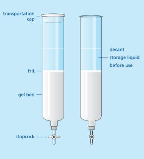
Allow the column to warm to ambient temperature if it has been refrigerated. Check to ensure the stopcock is in the closed position. Carefully remove the transportation cap from the top of the CentriPure N300 column and decant the storage liquid above the upper frit into a suitable waste reservoir.\*
