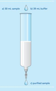
Carefully and evenly transfer a 30 mL sample onto the top of the upper frit. Allow the sample to completely enter the gel bed. Some eluent will flow out of the column and this can be discarded.
