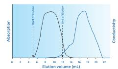
Elution profile overlay of albumin (5 mg OvA, black line – 280 nm) and free dye (2.5 µmol FAM, orange line – 490 nm) in DMSO/NaHCO<sub>3</sub>, elution with water (5 mL sample volume)
