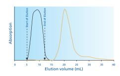
Desalting of protein solution (5 mg albumin (OvA) in 5 mL 0.8 M NaCl), elution with water
