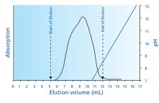
Separation of conc. ammonia and oligonucleotide after cleavage from solid support and removal of protecting groups (18-mer, Scale: 1 µmol, 5 mL sample volume)
