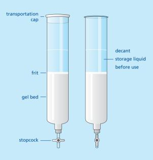
Allow the column to warm to ambient temperature if it has been refrigerated. Check to ensure the stopcock is in the closed position. Carefully remove the transparent transportation cap from the top of the CentriPure 1000 column and decant the storage liquid above the upper frit into a suitable waste reservoir.\*
