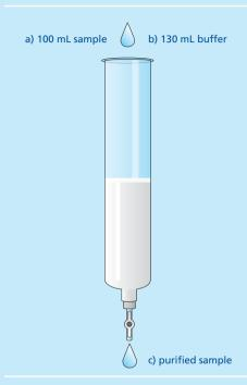
Carefully and evenly transfer a 100 mL sample onto the top of the upper frit. Allow the sample to completely enter the gel bed. Some eluent will flow out of the column and this can be discarded.
