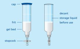
Allow the column to warm to ambient temperature if it has been refrigerated. Check to ensure the stopcock is in the closed position. Carefully remove the blue cap from the top of the CentriPure 200 column. Decant the storage liquid above the upper frit into a suitable waste reservoir.\*
