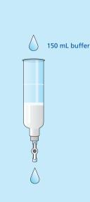
Ensure that the stopcock remains continuously in the open position during sample processing. The column is designed for the flow to stop after all fluid has entered the gel bed with no fluid above the upper frit. There is no need to close the stopcock during sample processing.
