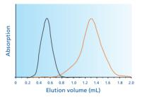
Elution profile overlay of ovalbumin (1 mg/mL) and free dye (TAMRA, 0,1 μmol) in a 200 μL sample volume.
