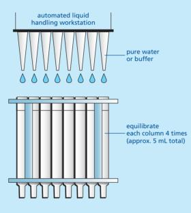
Choose a buffer for your specific application and use this same buffer for both equilibration and elution steps. To equilibrate the column, allow the buffer to enter the gel bed completely and to drain into a suitable waste reservoir.
