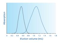
Desalting of protein solution (1 mg albumin (OvA) in 1 mL 0.8 M NaCl), elution with water (200 µL sample volume)
