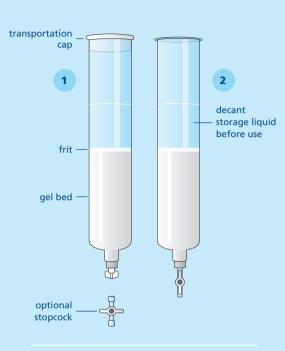
Allow the column to warm to ambient temperature if it has been refrigerated. Carefully remove the transparent transportation cap from the top of the CentriPure 1000 column and decant the storage liquid above the upper frit into a suitable waste reservoir.\*
