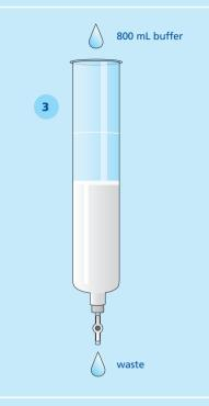
Ensure that the stopcock remains continuously in the open position during sample processing. The column is designed for the flow to stop after all fluid has entered the gel bed with no fluid above the upper frit. There is no need to close the stopcock during sample processing.
