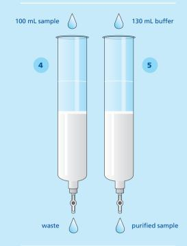
Carefully and evenly transfer a 100 mL sample onto the top of the upper frit. Allow the sample to completely enter the gel bed. Some eluent will flow out of the column and this can be discarded.
