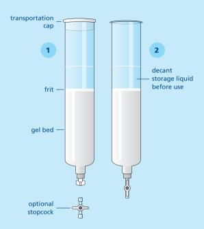
Allow the column to warm to ambient temperature if it has been refrigerated. Carefully remove the white cap for secure transportation from the top of the CentriPure 1500 column and decant the storage liquid above the upper frit into a suitable waste reservoir.\*
