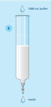
Ensure that the stopcock remains continuously in the open position during sample processing. The column is designed for the flow to stop after all fluid has entered the gel bed with no fluid above the upper frit. There is no need to close the stopcock during sample processing.
