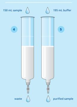
Carefully and evenly transfer a 150 mL sample onto the top of the upper frit. Allow the sample to completely enter the gel bed. Some eluent will flow out of the column and this can be discarded.
