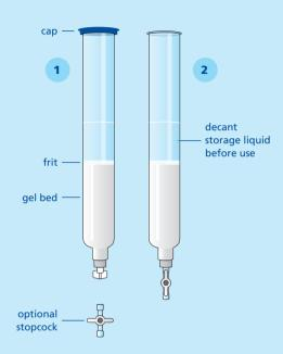
Allow the column to warm to ambient temperature if it has been refrigerated. Carefully remove the blue cap from the top of the CentriPure 400 column. Decant the storage liquid above the upper frit into a suitable waste reservoir.\*
