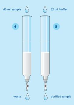
Carefully and evenly transfer a 40 mL sample onto the top of the upper frit. Allow the sample to completely enter the gel bed. Some eluent will flow out of the column and this can be discarded.
