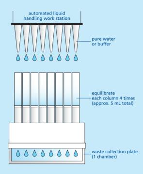
Choose a buffer for your specific application and use this same buffer for both equilibration and elution steps. To equilibrate the column, allow the buffer to enter the gel bed completely and to drain into the waste collection plate.
