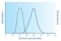
1.0 mL sample volume Anti-rabbit IgG, 1 mg: black line (280 nm) NaCl, 0.8 M: blue line (µS/cm) Elution with pure water
