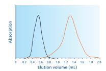
Elution profile overlay of ovalbumin (1 mg/mL) and free dye (TAMRA, 0,1  $\mu mol)$  in a 200  $\mu L$  sample volume.
