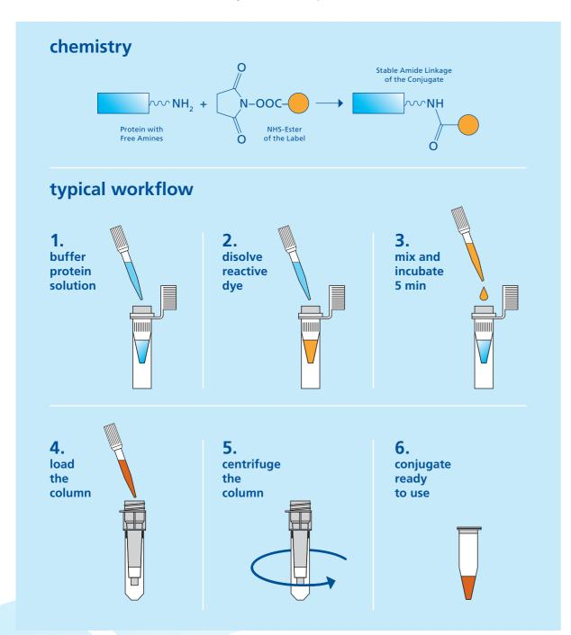
Delivers precision labeling and rapid purification of antibodies, enzymes and other proteins. For controlled labeling and purification of proteins having a molecular weight greater than 25 kDa.
