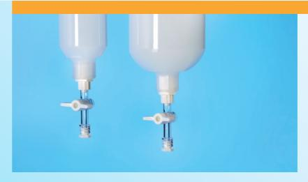
CentriPure Gel Filtration Columns are specifically designed for rapid and efficient removal of small molecules (dyes, salts, biotin, haptens, etc.) from larger proteins, nucleic acids, or nanoparticles, which are simultaneously purified and desalted in a single step.
